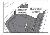
3 Close the transmittance specimen chamber cover.
