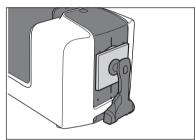
3 Position the specimen so that the part you want to measure is within the measurement points.
