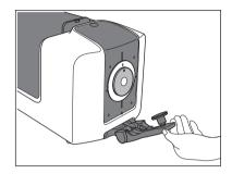
2 As shown in the figure, press on the sample holder so that the sample holder fits into the indentation on the reverse side of the gloss calibration plate.
